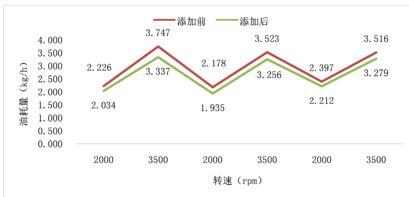
Figure 10. Diagram of comparison of fuel consumption in engine dual idle condition test 图 10. 发动机双怠速工况试验油耗量对比
