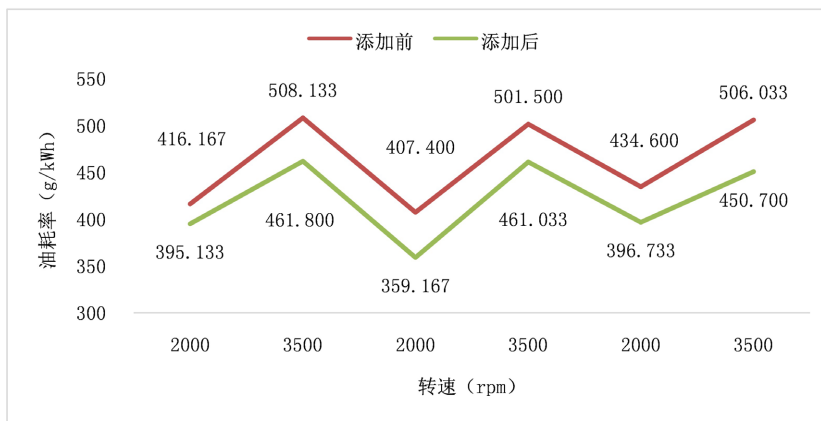
Figure 11. Diagram of comparison of fuel consumption rate in engine dual idle condition test 图 11. 发动机双怠速工况试验油耗率对比
