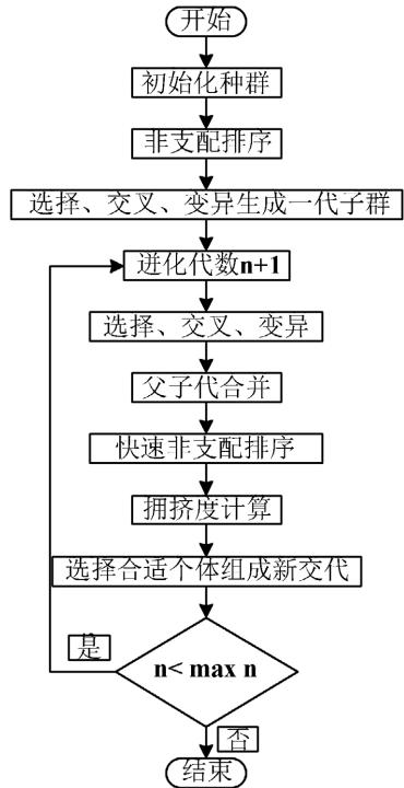
**Figure 3.** Flowchart of NSGA-II Algorithm
