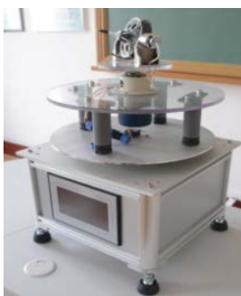
Figure 3. Single-axis stabilized platform teaching AIDS
