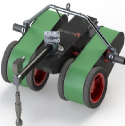
Figure 10. MW-SR-01 swinging arm ship derusting robot
