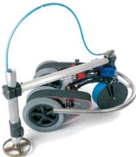
Figure 7. RJE-1000 ship cleaning robot
