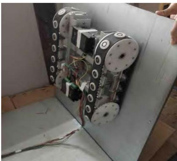
**Figure 12.** A new electromagnetic adsorption wall-climbing robot
