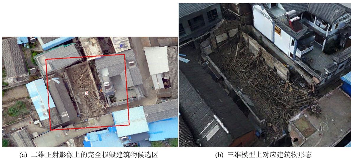
Figure 7. Candidate areas for completely damaged building that are easily identified by 2D orthophotos
