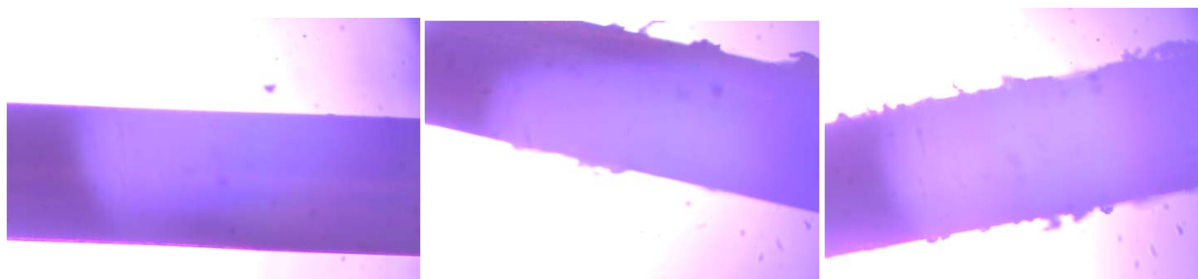
Figure 10. The micrographs of copper wire after sanding. From left to right: sanding 0, 1, 2 time (s)
