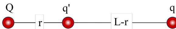
Figure 2. A linear network composed of three point charges 图 2. 三个点电荷组成的线型网络
