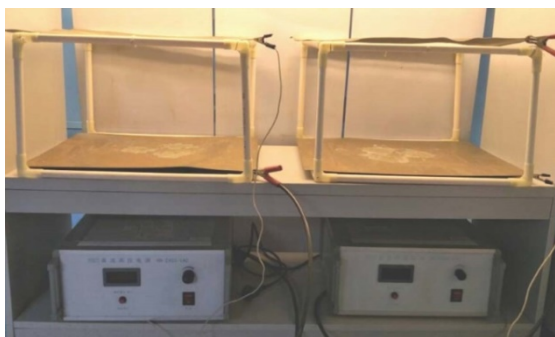
Figure 1. High-voltage electrostatic field device (Left: Negative high-voltage (-/+) electrostatic field; Right: Positive high voltage (+/-) electrostatic field)
