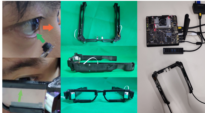
Figure 2. Hardware environment with OST-HMD and TX2 图 2. 光学头戴式显示器和 TX2 的硬件设备
