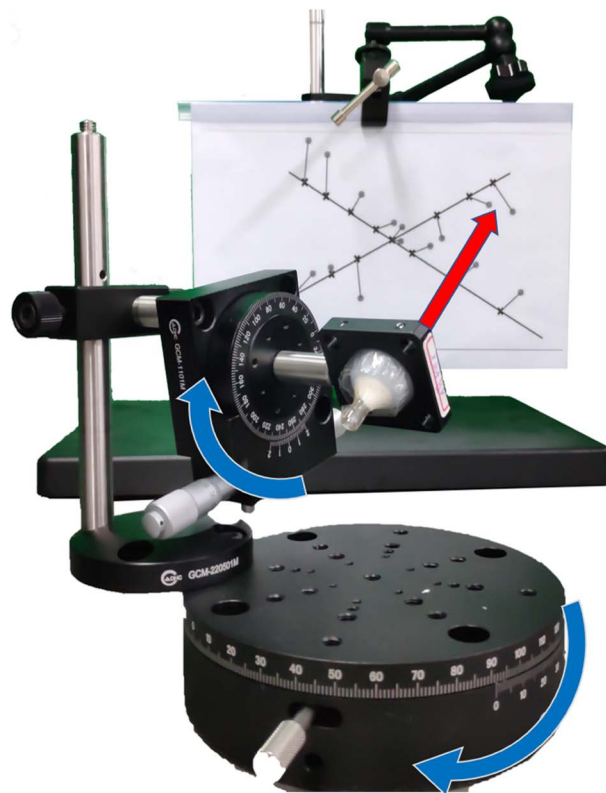
Figure 5. Error measurement hardware 图 5. 误差测量实物图
