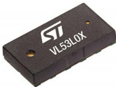
Figure 4. Package diagram of VL53L0X chip
