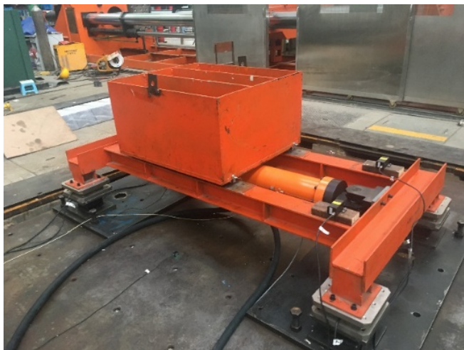
Figure 3. Physical diagram of electro-hydraulic servo AMD system 图 3. 电液伺服 AMD 系统实物图
