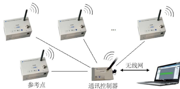
Figure 3. The wireless ambient excitation modal test system models for DH5907A
