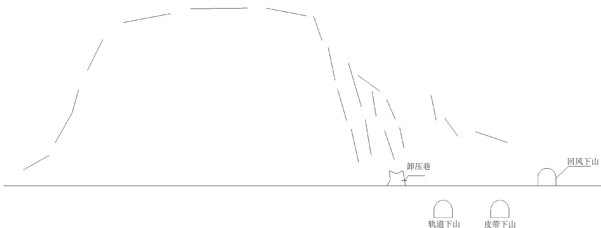
Figure 10. Main fissures of rock strata around pressure relief roadway
