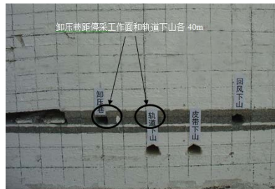
Figure 6. Specific location of pressure relief roadway
