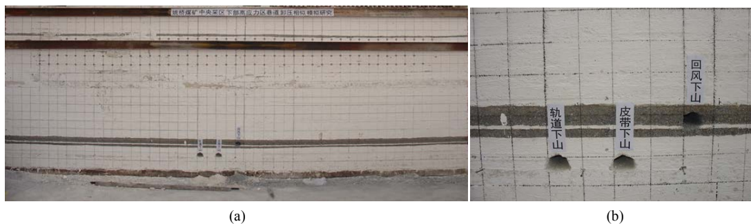
Figure 2. Location of centralized downhill of 7011 mining area. (a) Similar material model; (b) Roadway location 图 2. 7011 采区集中下山位置图。(a)相似材料模型；(b)巷道位置
