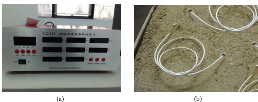
Figure 1. Stress monitoring of model rock. (a) Comprehensive tester; (b) Micro force sensor
