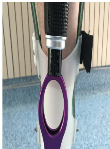
Figure 4. Displacement and weight-limiting device of rehabilitation brace after lower limb fracture operation
