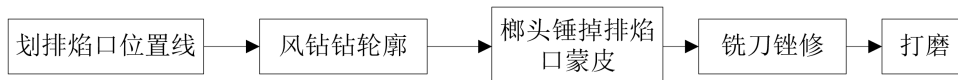
Figure 2. Flow chart of traditional production process of drain port 图 2. 排焰口的传统制作工艺流程图
