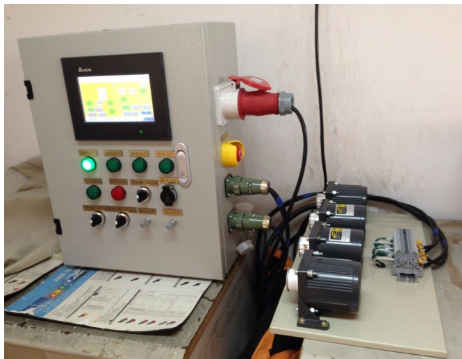
Figure 1. The integrated intelligent fire protection inspection control device 图 1. 智能一体化消防巡检控制装置
