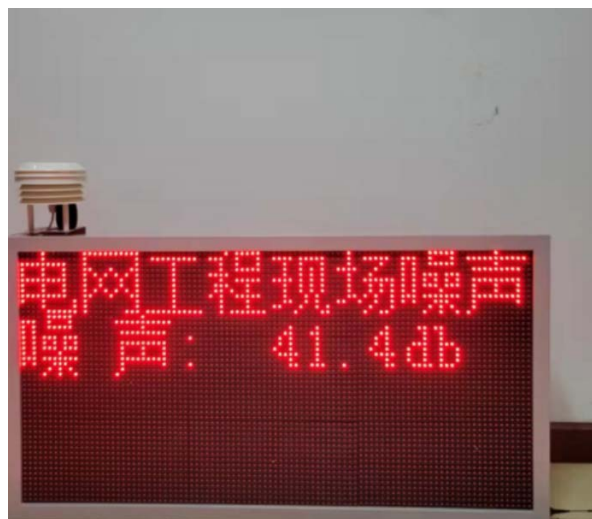
Figure 2. Schematic diagram of on-site noise detection of power grid transmission and transformation projects 图 2. 1/3 电网输变电工程现场噪声检测示意图
