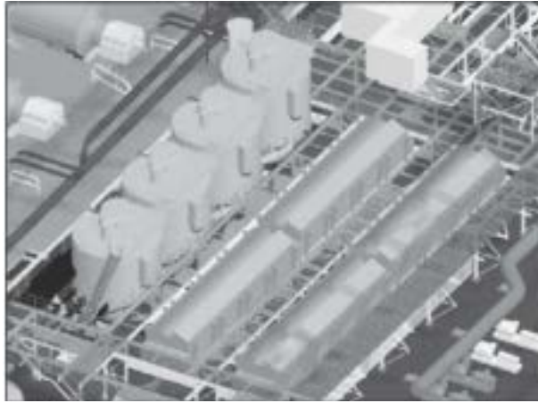
Figure 2. The second stage had been completed, the new flotation cells and the old flotation cells were working together 图 2. 第二阶段完成，新浮选槽与旧浮选槽一起工作的模型
