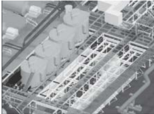
Figure 3. After the old flotation cells were shut down and dismantled, the existing steel structure had replaced the layout 图 3. 旧浮选槽停产并拆除后，现有的钢结构已取代布置
