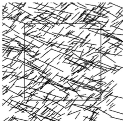
Figure 3. Two sets of cracks generated by Monte-Carlo method
