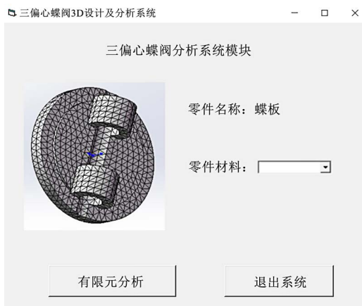
Figure 10. Finite element analysis interface of triple eccentric butterfly valve 图 10. 三偏心蝶阀有限元分析界面
