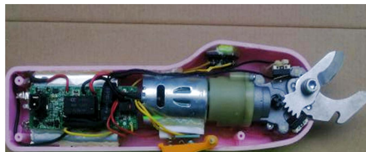
Figure 7. Physical internal structure of the pruner
