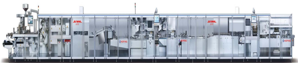
Figure 5. Physical prototype of blister dual-track sleeper wrapping and flow box packing machine 图 5. 泡罩双轨枕包含流装盒一体机实物样机
