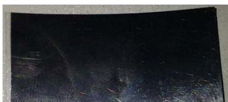
Figure 3. Sputtered Ni thin film sample under the conditions of magnetic field
