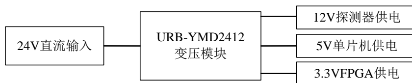
Figure 5. Structure of power source module
