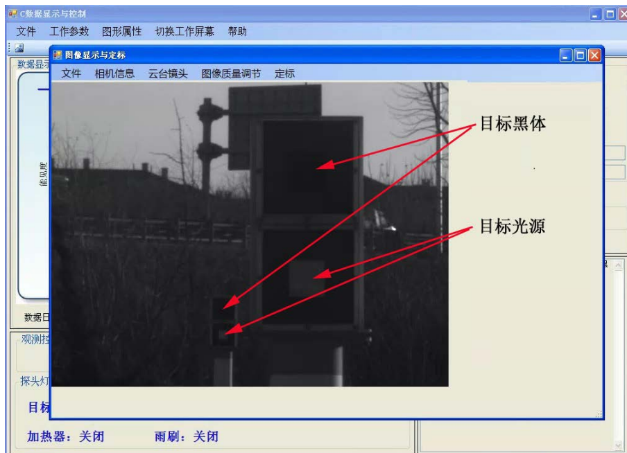
Figure 2. Video window of atmospheric visibility observation system (not calibrated) 图 2. 大气能见度观测系统的视频窗口(未定标)
