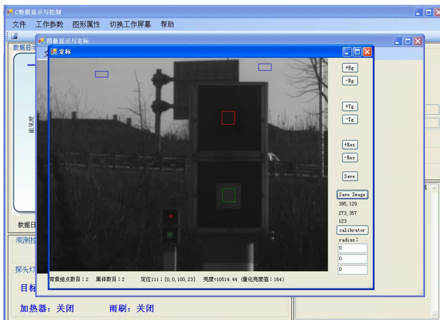
Figure 3. Video window of atmospheric visibility observation system (calibrated, blue box for sky positioning)
