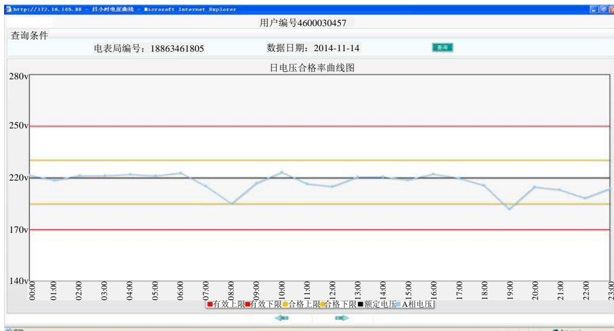
Figure 1. The end of the line a user voltage curve (before the governance)
