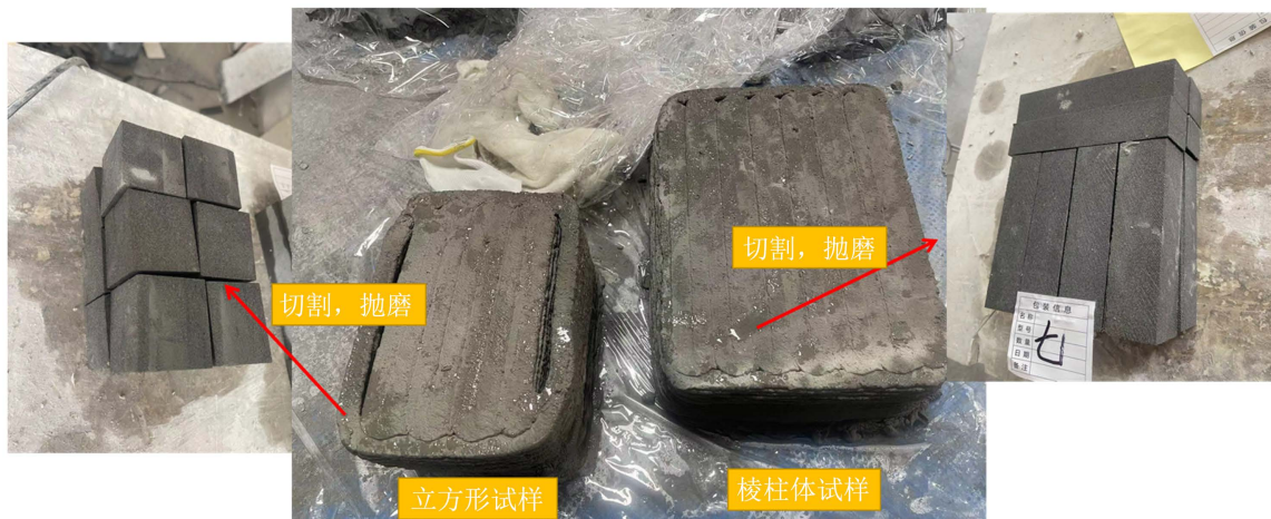
Figure 3. 3D printing antimony tailings UHPC sample 图 3. 3D 打印锑尾矿 UHPC 试样
