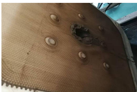
Figure 4. Typical filter cloth state diagram after mud discharge
