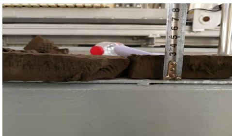
Figure 2. Schematic diagram of filter cake thickness on the 9th day
