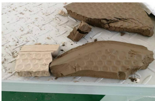
Figure 3. Schematic diagram of mud cake moisture content on the 9th day
