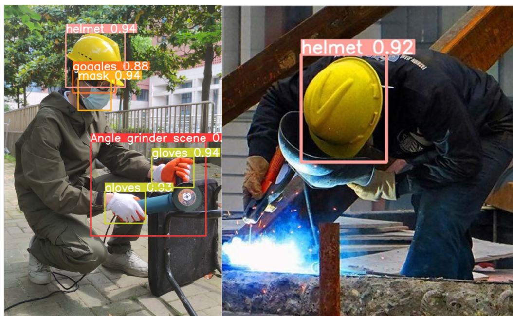
Figure 3. Inspection results (the picture on the left shows the operation of an angle Grinder, the picture on the right shows the operation of a non-angle grinder)
