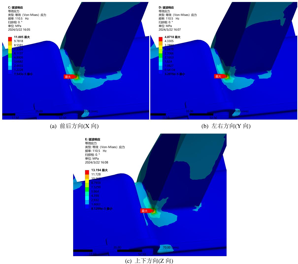
**Figure 5.** Equivalent stress cloud map with a frequency response of 110.5 Hz
