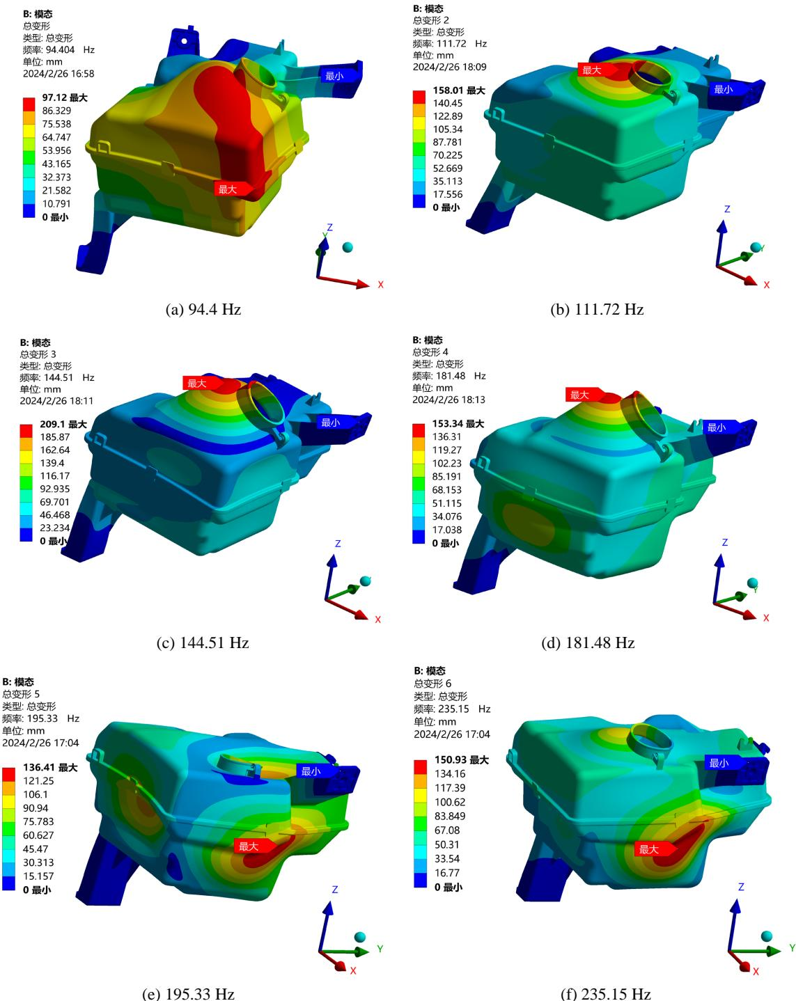
**Figure 3.** Cloud map of the first six natural frequencies and modes of the washer reservoir
