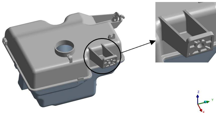
**Figure 7.** Structural improvement of bracket A
