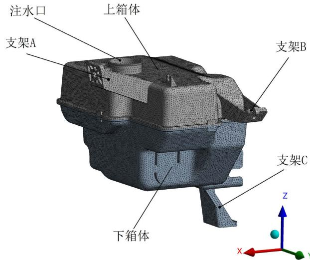
**Figure 1.** Finite element model of washer reservoir
