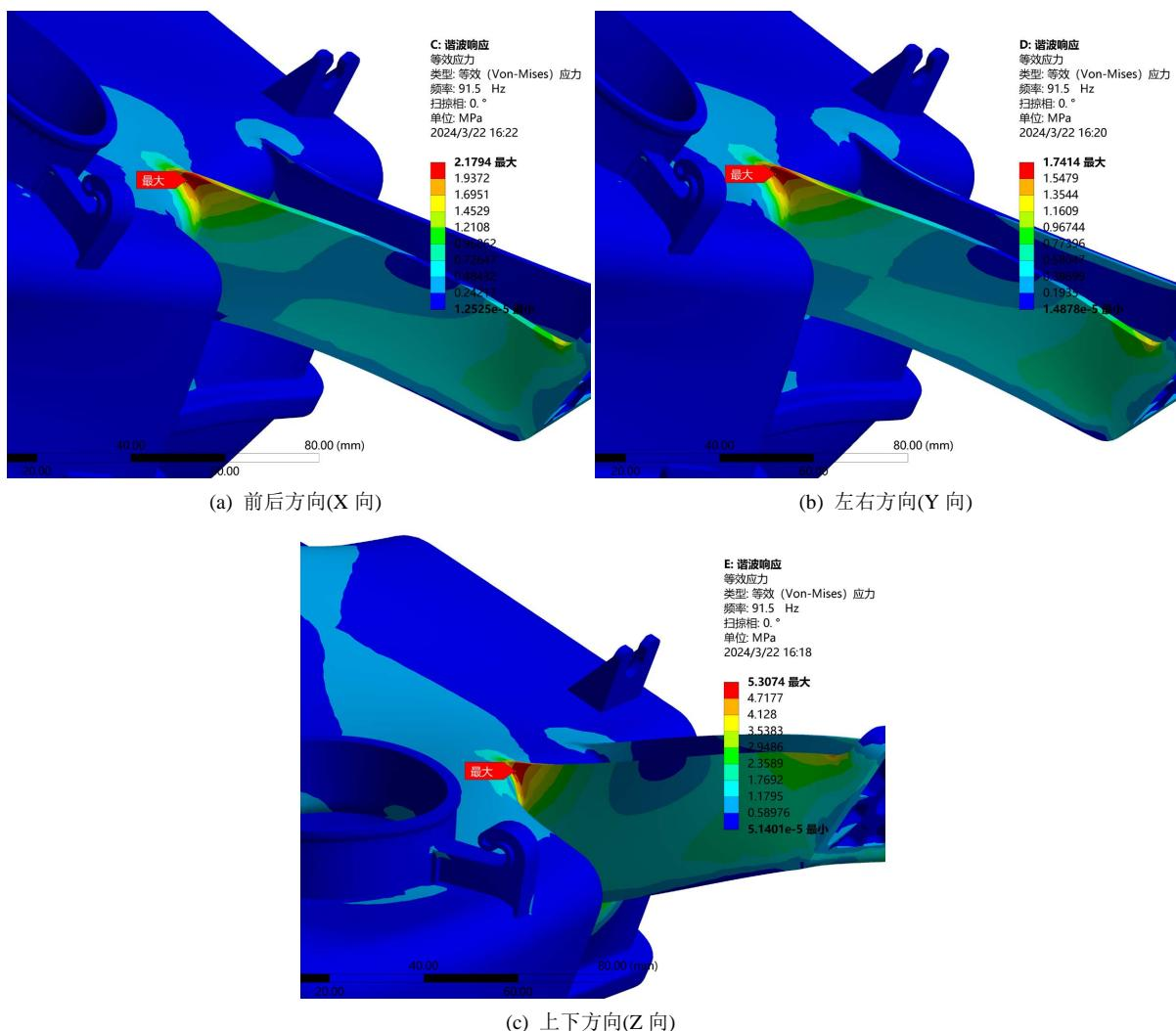
**Figure 4.** Equivalent stress cloud map with a frequency response of 91.5 Hz
