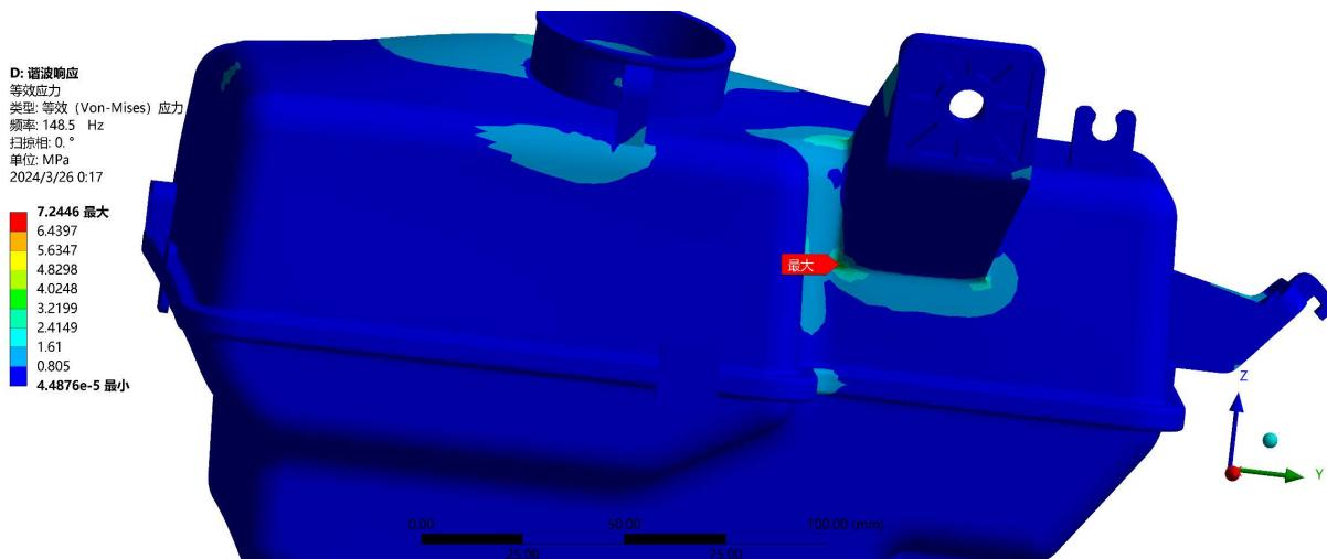
**Figure 8.** The maximum stress value of bracket A after improvement
