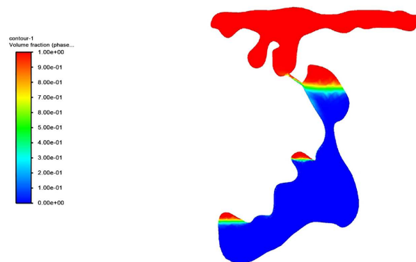
Figure 16. Water is injected at the bottom of the lower karst cave and oil is extracted from the surface 图 16. 下溶洞底部注表层采
