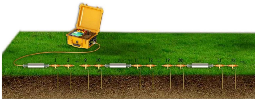
Figure 3. Distributed high-density resistivity instrument
