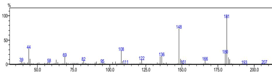
Figure 6. The mass spectra of 2-(Methylthio) benzothiazole
