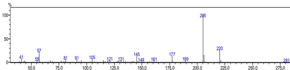
Figure 5. The mass spectra of 2,6-Di-tert-butyl-4-methylphenol (BHT)
