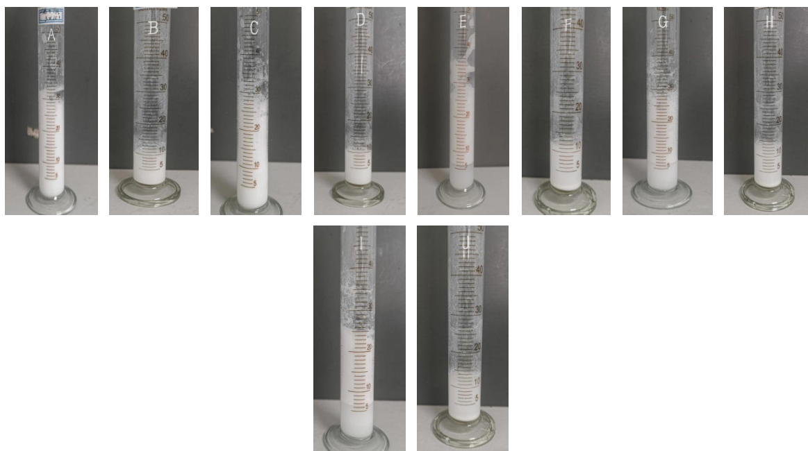
Figure 6. Cycling between defoaming and foaming of a dispersion of 0.5 % \text{TiO}_2 nanoparticles in 3 \times 10^{-4} mol/L CTAB aqueous solution by adding equal moles of SDS and 3 \times 10^{-4} mol/L free CTAB (0.1g solution in 3 \times 10^{-2} mol/L) alternatively. The photographs were taken 10 min after shaking
