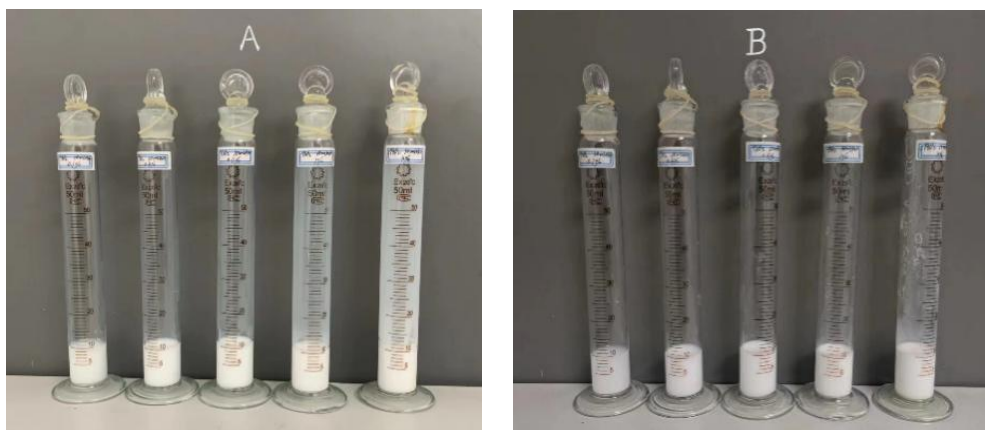
Figure 2. Digital photographs of aqueous foams stabilized by TiO 2 nanoparticles alone at different concentrations, taken immediately (A) and 24 h later (B) TiO 2 nanoparticles concentrations from left to right are 0.1%, 0.3%, 0.5%, 1%, 2%
