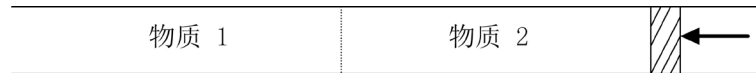
Figure 2. Shock tube with a moving piston 图 2. 带移动活塞的激波管问题
