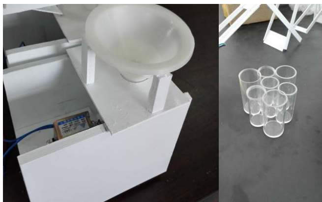
Figure 7. Packing mechanism for coins 图 7. 硬币包装机构
