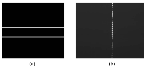
Figure 3. (a) Double-slit pattern; (b) Its Fourier spectrum 图 3. (a) 双缝图样; (b) 双缝图样的傅里叶频谱
