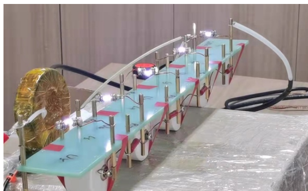
Figure 6. The discharge moment of Marx generator to a resistor
