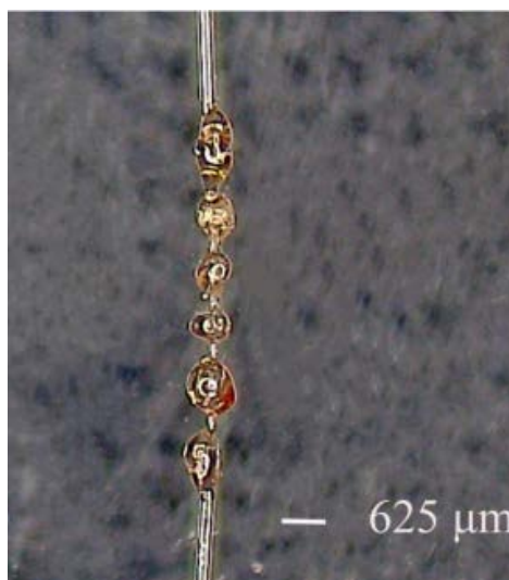
Figure 1. Sugar-coated gourd type optical fiber thermometer
