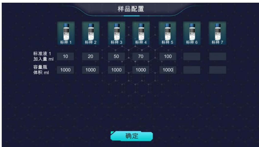
Figure 2. Virtual simulation gas chromatography standard solution configuration
