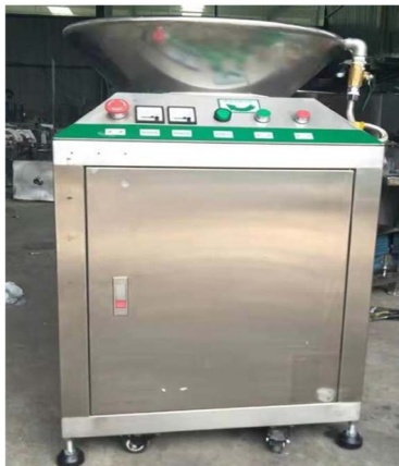
Figure 2. Kitchen waste crushing and dewatering machine (Pictures from the Internet) 图 2. 餐厨垃圾粉碎脱水处理一体机(图片来源于网络)
