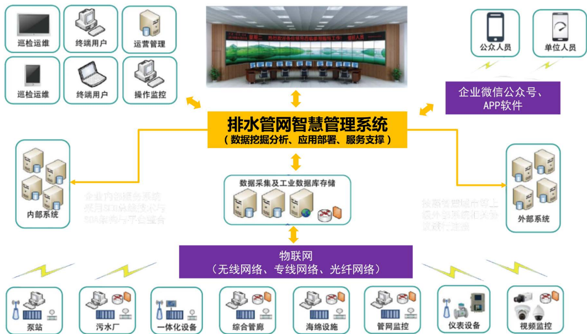
Figure 1. Image connection diagram of drainage network intelligent management system facilities
