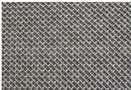
Figure 4. Third generation of metal fiber filter material 图 4. 第三代金属纤维滤料
