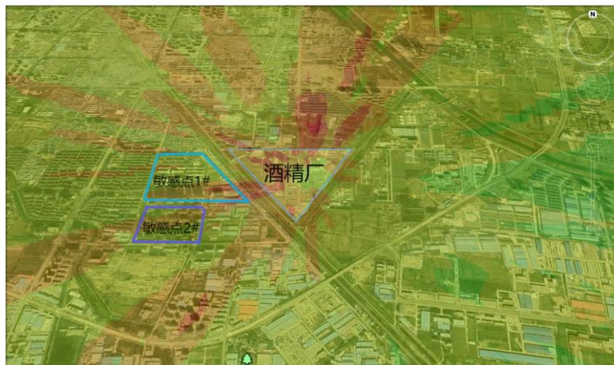
**Figure 4.** Overall exposure influence around 2 km around alcohol plant (maximum annual odour concentration in hour)
