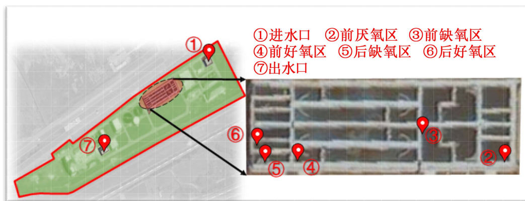
Figure 2. Improved A 2 /O process sampling point distribution diagram
