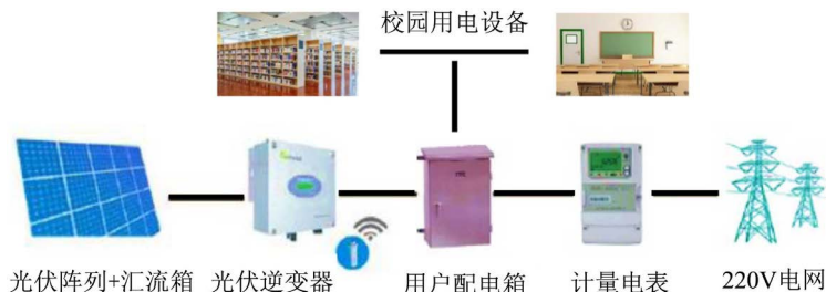
Figure 1. Schematic diagram of campus Dis-PV power system
