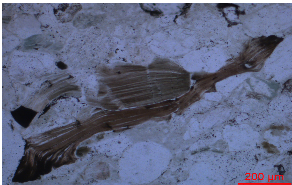
Figure 8. Chlorite presents biotite illusion distributing among debris particles 图 8. 绿泥石呈黑云母假象分布于碎屑物颗粒之间
