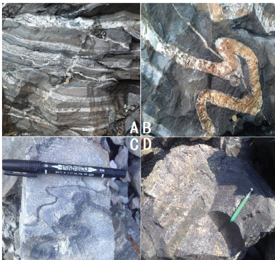
A——一条带状磁铁矿石英岩；B——磁铁矿石英岩石英肠状构造；C——磁铁矿内受剪切作用呈“S”形褶皱构造；D——磁铁矿石英岩发育褶皱变形。A—banded magnetite quartzite; B—intestinal structure; C—“S” fold structure; D—folding deformation.
