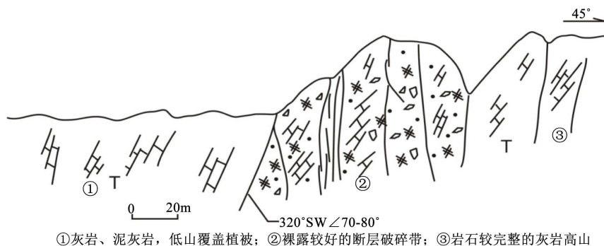
Figure 4. Geology section of Daju fault near Zongsi
