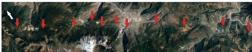
Figure 5. Satellite image interpretation of the Majiacun-Daju section of Daju fault
