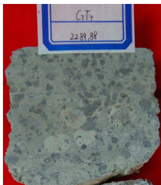
Figure 4. Gravel limestone core diagram of well Qi626-2
